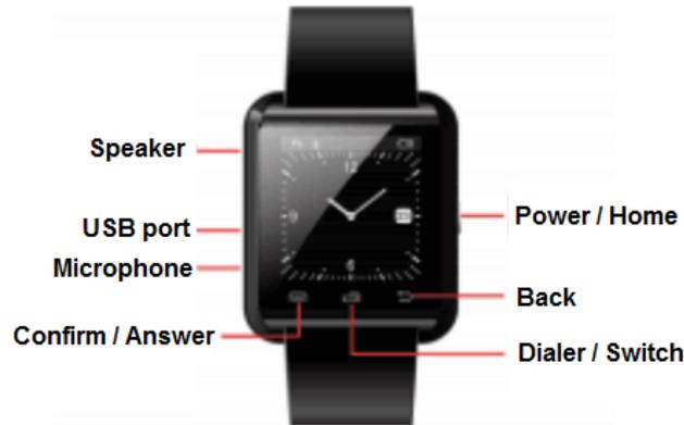
Power/ Home : Long press to start or turn power on/off, short press to return to the standby interface.
