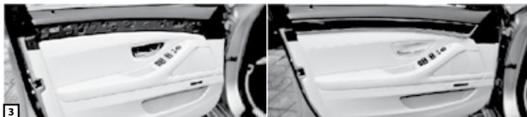
Finally, reconnect the wirings and door latch cables, reassemble the removed parts back on to the door and tighten the door panel's screw firmly
