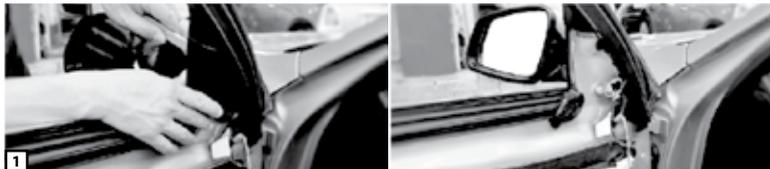
Carefully remove original tweeter housing. (Wind down window for easy installation)
