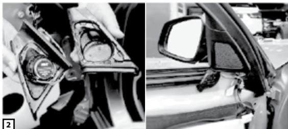
Replace the tweeter and insert the foam to the triangle housing. (Door triangle housing has speaker grill and holder for tweeter which is not included in the Blaupunkt speaker)
