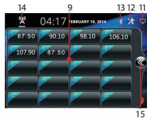
1. Touch to start searching the radio frequency & storing the strongest signal station into memory. After one cycle searcher, the unit starts into broadcasting of the present memory stations for a few seconds. Touch again to stop this intro broadcasting.
