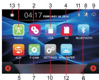
Touch the icon on the desired mode on screen and the unit will then enter into the mode that you selected for operation. Hold & slide on the lower portion of the screen (input icons) to shift to other the **MAIN MENU** that shows the hidden input or operation icons.
