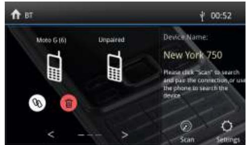
After pressed, the unit will display a screen listing paired devices. Press the [🔗] icon to reconnect a previously paired phone to the BT radio. Press the [🗑️] icon to unpair the phone from the unit.
