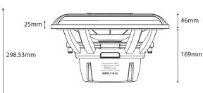
Nominal SD: 598cm<sup>2</sup> RMS handling: 1000 Impedance:  $2\Omega+2\Omega$
