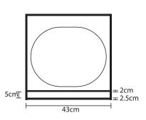
\*All enclosure dimensions are internal and include basket displacement. The above enclosure shape is an example and these dimensions can be modified provided that the exact internal volume is retained 1-inch thick M.D.F is recommended as a minimum
