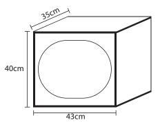
\*All enclosure recommended dimensions are for internal dimensions only. The above enclosure shape is an example and these dimensions can be modified provided that the exact internal volume is with minimum of 1" M.D.F thickness.
