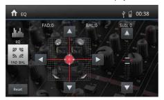
Adjust fader and balance with  $[ \triangledown ] / [ \blacktriangle ]$  or  $[ \blacktriangleleft 1/[ \blacktriangleright 1]$ .
