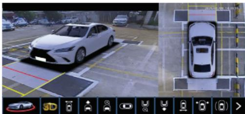
c) When the result of the automatic stitching is not ideal, you can enter the lens correction section, and perform lens correction on the four cameras of the front, rear, left, and right.
