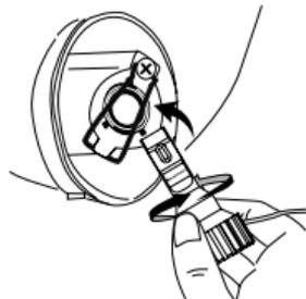
4. Please ensure the diodes (LED chips) of headlamp are in a side to side orientation.
