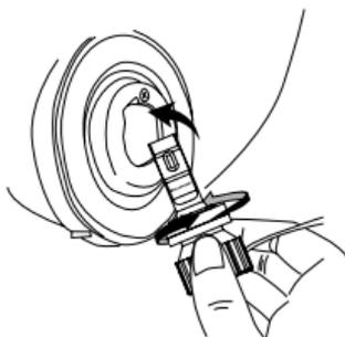
2. Please ensure the diodes (LED chips) of headlamp are in a side to side orientation.
