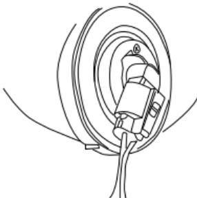
3. Remove the halogen bulb from headlight housing.
