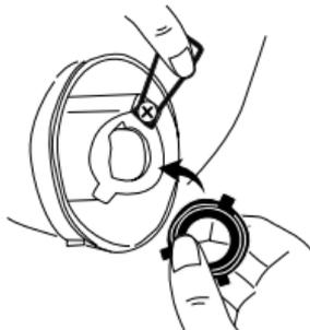
3. Install the headlamp into headlight housing and turn clockwise to secure it.
