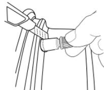
2. Install & adjust the valve sensor onto the wheel barrel. Screw & tighten the nut & valve.
