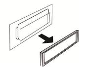
3. Insert the keys supplied on the both sides of the unit until they click. Pulling the keys and makes them to remove the unit from the dashboard.
