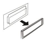
3. Insert the keys supplied on the both sides of the unit until they click. Pulling the keys and makes them to remove the unit from the dashboard.
