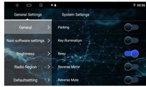
Parking – In Parking "On" mode, the screen will display Warning information if you play video. The warning screen will prevent the driver from watching videos while the vehicle is in motion.
