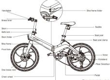
Blaupunkt Rear hub motor, DC 36 V/ 350 W, 50 Nm, IP54, brushless, maintenance free 36 V/ 10,5 Ah LG- Lithium- Ion battery w. integrated BMS 36 V/ 15 A DC Cadence & speed sensor 3 levels of peddle and throttle assist. Throttle with walk mode and speed control. LC- Display wit 3 function keys, backlight. Functions: Speed, ODO, TRIP, TIME, PAS LEVEL, battery, LED light, auto power off, error display. Switching power supply (AC 100 – 240 Volt), 42 V, 2 A Approx. 4- 6 h Up 44 miles max. 20 MPH
