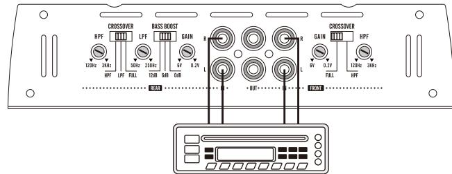
system 3: 2 channel bridged connection
