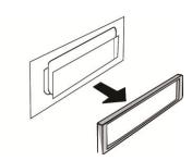
3. Insert the keys supplied on the both sides of the unit until they click. Pulling the keys and makes them to remove the unit from the dashboard.
