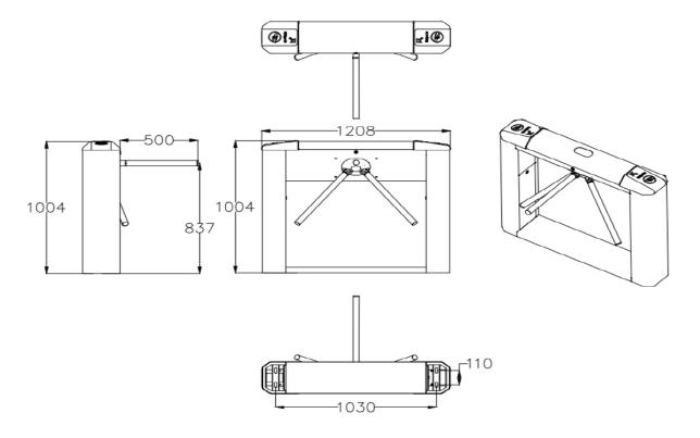
**Note:** This model can be freely combined into single-channel, dual-channel, and multi-channel. The standard passage width of this model is 550mm.
