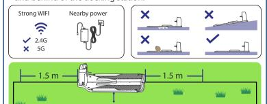
Warning: Please place the docking station on a flat and soft surface to ensure that the 40 cm long metal ground nails can be smoothly inserted into the ground. Watch for underground pipes.
